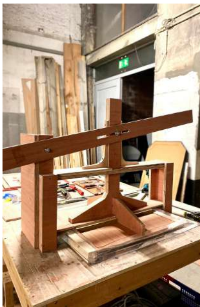
Fig.23 - The press to maintain substrates dense enough into the mold
