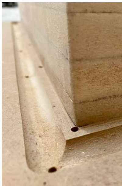
Fig.22 - A specific counter mold made to press the plastic mold for mycelium panels
