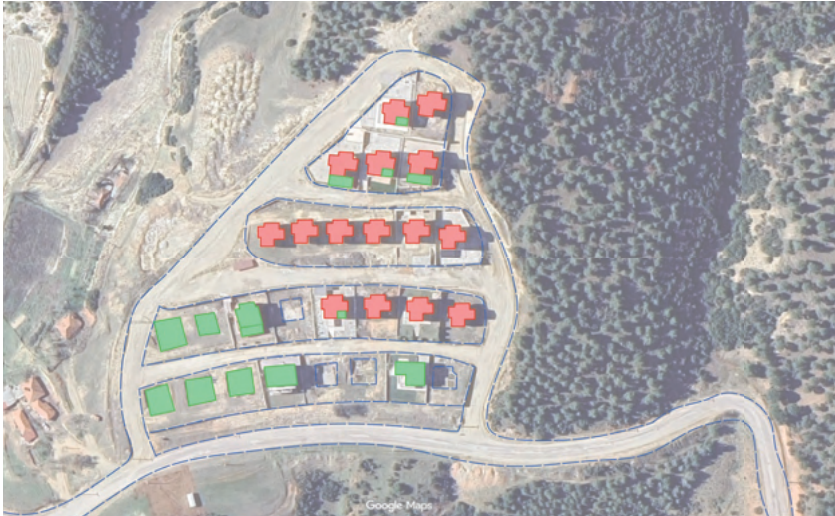
Fig. 5: Completed structures reveal ongoing modifications, often expanding beyond their original limits and altering the initial design. In the diagram, red indicates the original representation of buildings, while green shows later additions.
