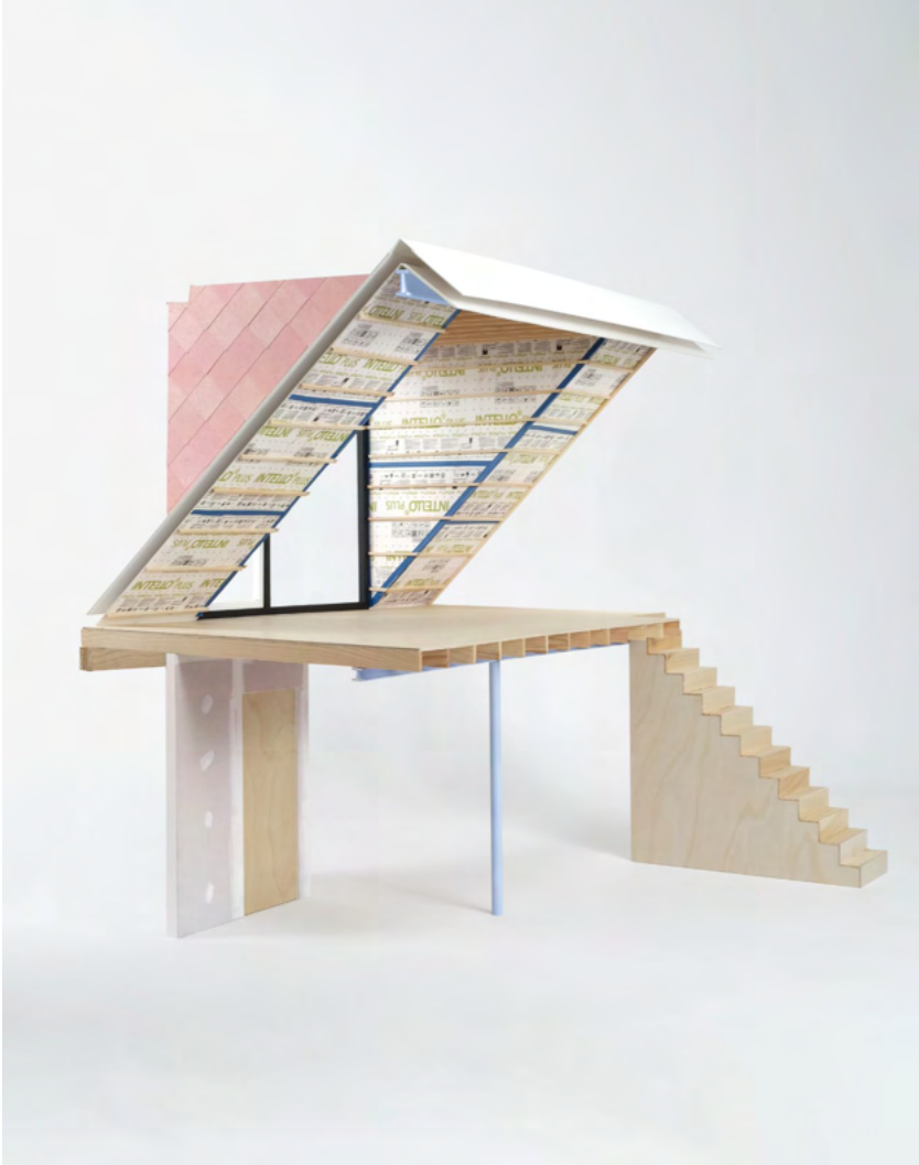
Study model of the Pont de Luttre project 1:10. Roof refurbishment and extension with the addition of a dormer and access to the roof terrace, limited to the scope of our intervention.
