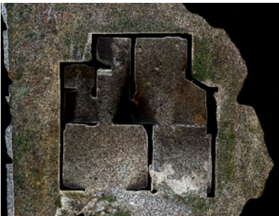
Fig. 4: Processed point cloud in CloudCompare showing the clear distinction between the building footprint and the surrounding ground surface.
