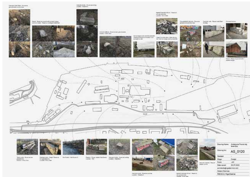
Pavement sketch about turning rubble from the territory into mosaics, which gave wheelchairs access to the industrial port. Below a mapping of rubble within the port that was used to discuss logistics for moving them around the territory.
