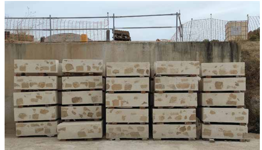
Precast concrete blocks mixed with recycled marès stone. Photo by Harquitectes
